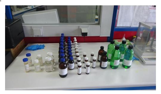
A tailored made groundwater sampling protocol was determined according to the clients' needs as well as a health and safety plan. Groundwater sampling were carried out by the low-flow sampling method (ASTM) and dedicated pre-preserved containers were used for each contaminant group. The samples were packed in coolers and shipped overnight to the laboratory. As soon as the analyses data were available, the conceptual site model was developed.
